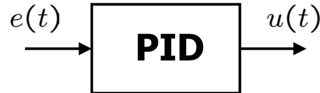
$$\begin{aligned} u(t) &= K_p \left[ e(t) + \frac{1}{T_i} \int_0^t e(\tau) d\tau + T_d \dot{e}(t) \right] \\ &= K_p e(t) + K_i \int_0^t e(\tau) d\tau + K_d \dot{e}(t) \end{aligned}$$
