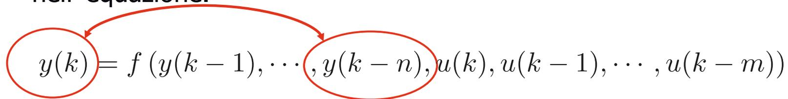
$$y(k) = f(y(k-1), \dots, y(k-n), u(k), u(k-1), \dots, u(k-m))$$
