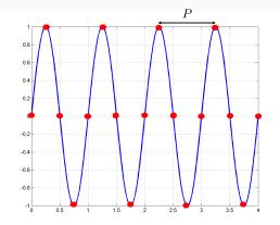
Reducing the sampling period (i.e. increasing the sampling frequency) the ambiguity disappears: no more frequency fold-over effect.
